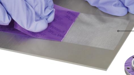
3M™ Anodization Masking Tape 8985L survives chromic acid with excellent masking lines and clean one-piece removal.
